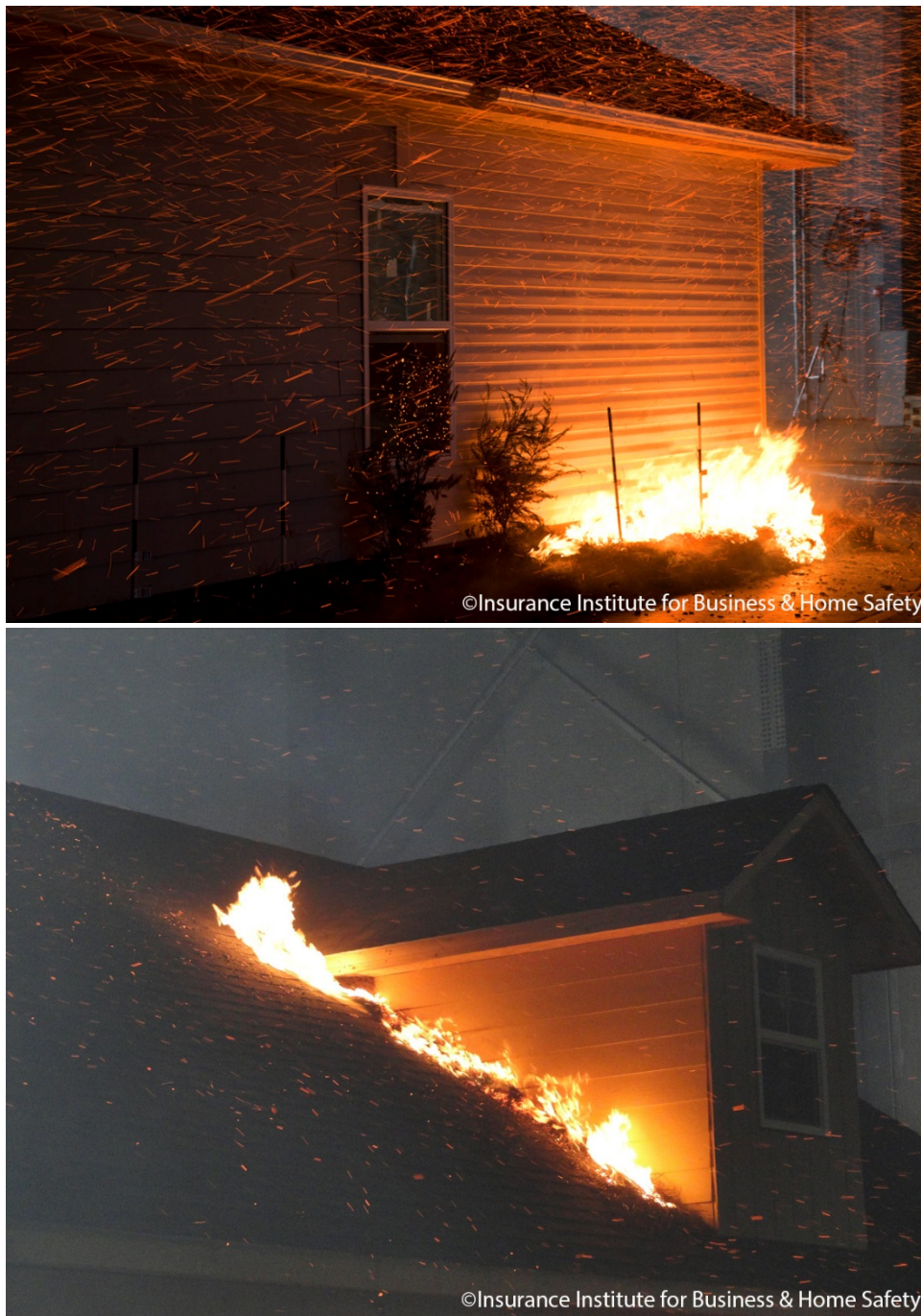
Figure 15. Ember ignitions of pine needle mulch at the base of an exterior wall (top) and pine needle debris at a roof-to-wall intersection (bottom). Photos are from experiments conducted at the IBHS Research Center in 2011.
