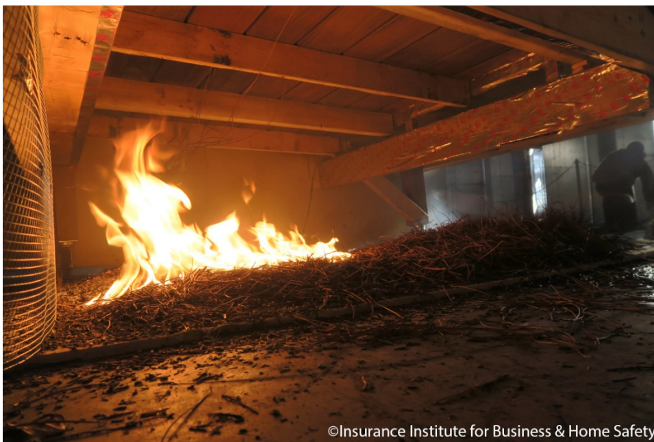
Figure 19. Ember penetration through gaps between deck boards; embers falling to ground (top) and resulting in the ignition of pine needles under deck (bottom).
