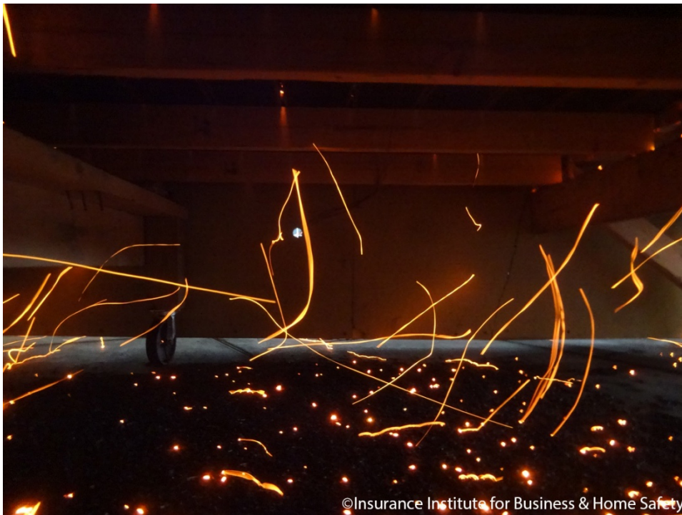
Figure 18. Ember penetration through gaps between deck boards and accumulating on the ground below.
