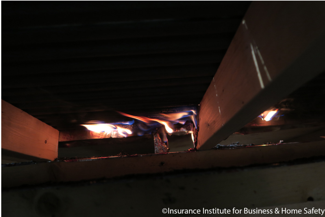
Figure 23. Flame spread in the underdeck area of PC product PE-1.
