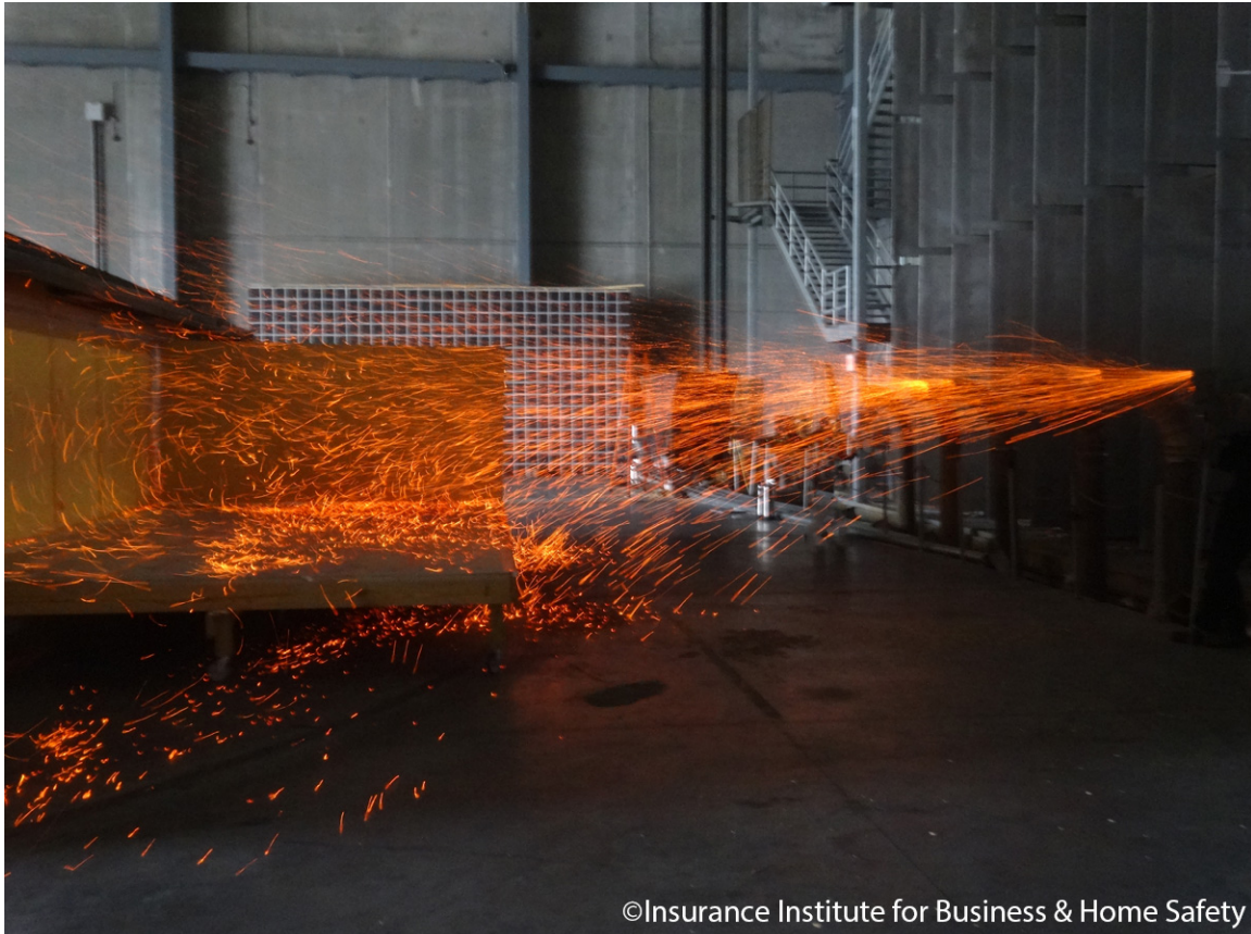
Figure 6. Test deck exposed to embers from ember generators.
