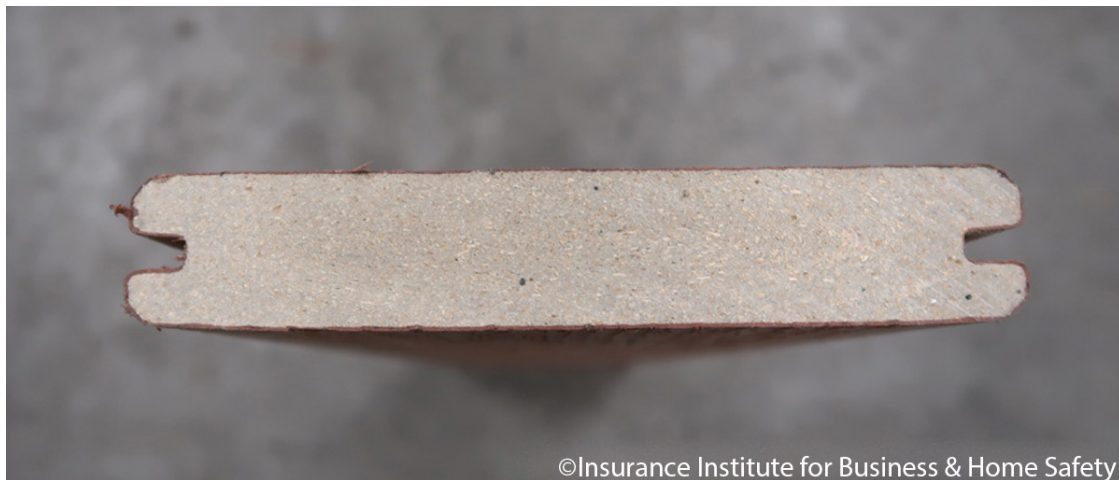
Figure 7. Example of a capped PC deck board. Note the reddish outer layer surrounding the lighter gray core material.
