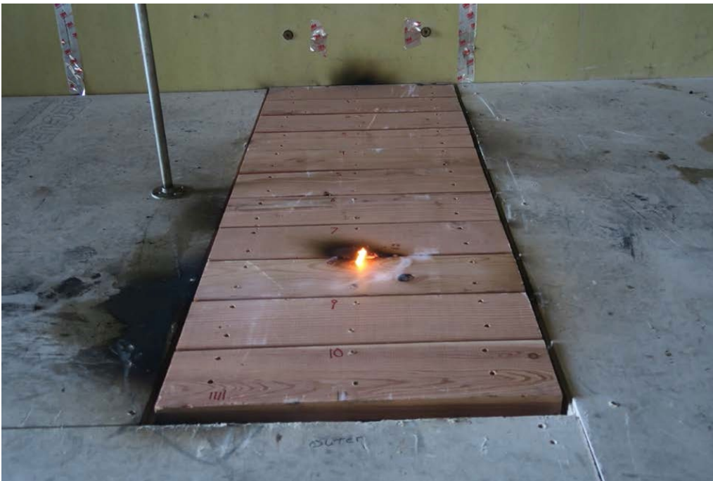
Figure 26. When deck boards were parallel to the building, fire would propagate laterally (parallel to the building) in the gap between deck boards, and toward the building at the interface between the bottom of the deck board and top of joist. Flaming combustion would occur when the fire reached a gap. Smoldering combustion would occur in the underdeck region when propagation was occurring in the interface between the top of a joist and bottom of a deck board.
