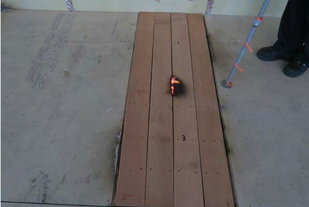
Figure 25. When deck boards were perpendicular to the building, fire spread toward the building occurred in the gap between deck boards.
