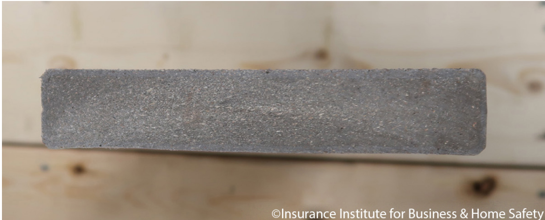
Figure 8. Example of a non-capped PC deck board.
