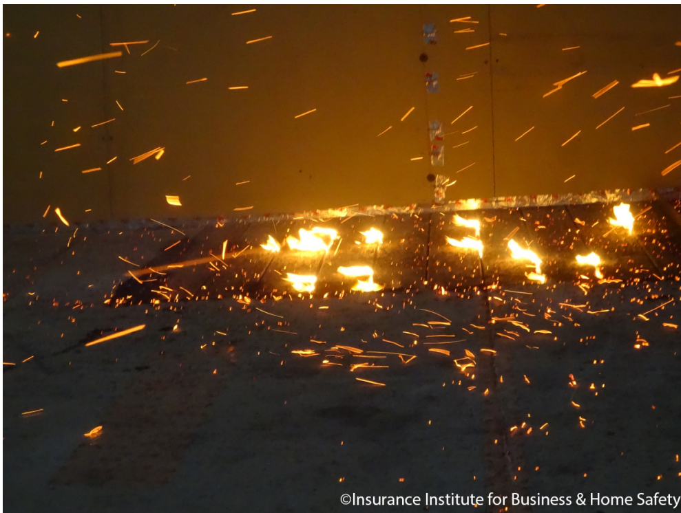
Figure 13. Flame heights (never more than a few inches high) on ignited, medium-density softwood deck. Flaming was sustained when there was sufficient heat transfer between components (i.e., deck boards and joists), after which flaming ceased.
