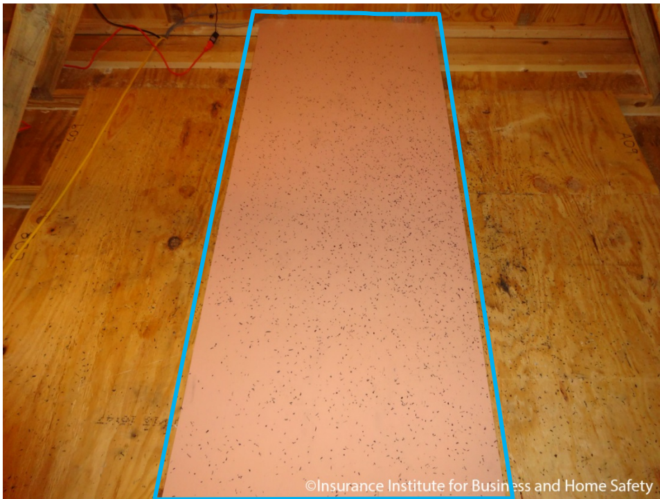
Figure 13. Embers that landed on the 3 ft by 8 ft (0.9 m x 2.4 m) panel (blocked in blue) were collected and weighed after each test. This technique provided means to quantify ember entry through the gable end vent. Note that embers (the black particles) landed on and off the panel. Only embers that landed and accumulated on the panel were weighed.
