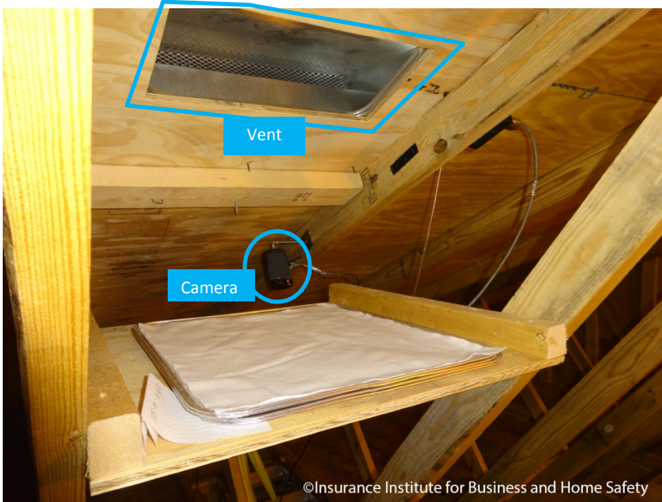
Figure 12. Typical video camera setup used to evaluate ember entry into a through-roof vent.
