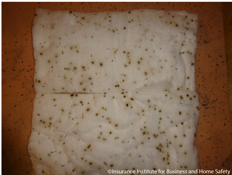
Figure 19. A cotton pad positioned on the attic floor at the base of a gable end vent showing numerous ember strikes. The cotton exhibited short-term smoldering combustion, but always self-extinguished without transitioning to flaming combustion.
