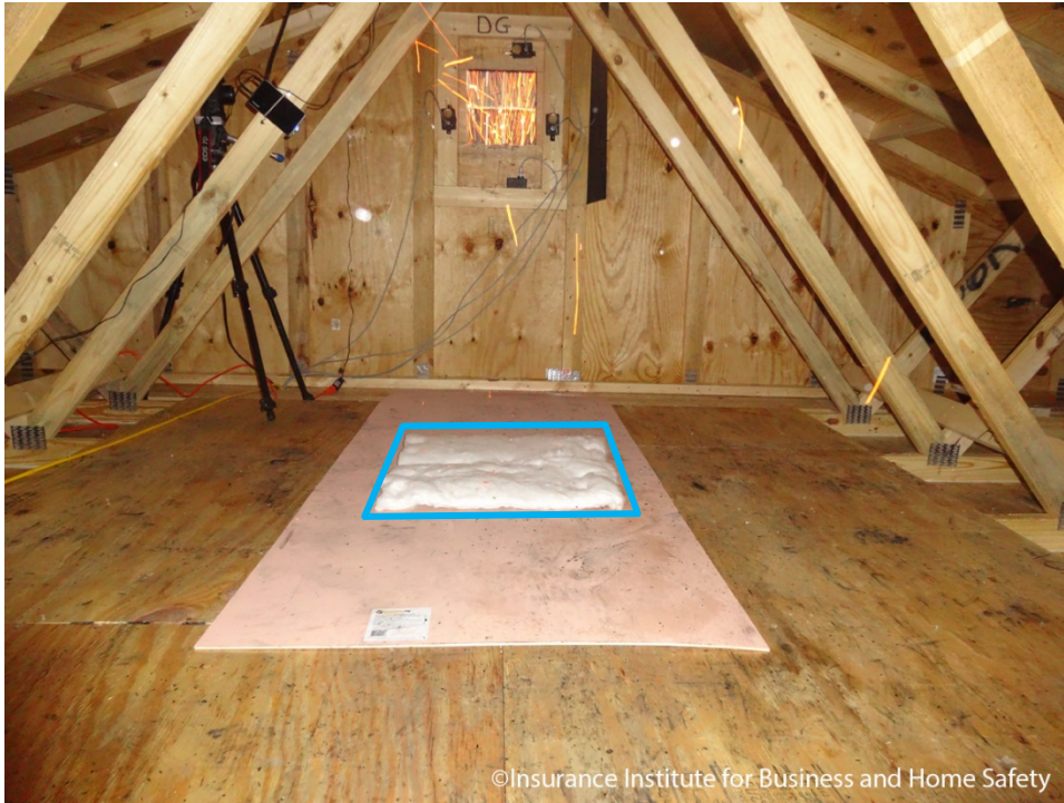
Figure 14. A cotton pad was placed on a horizontal surface, near the entrance of gable end and all through-roof vents to evaluate the ability of entering embers to ignite a combustible material.
