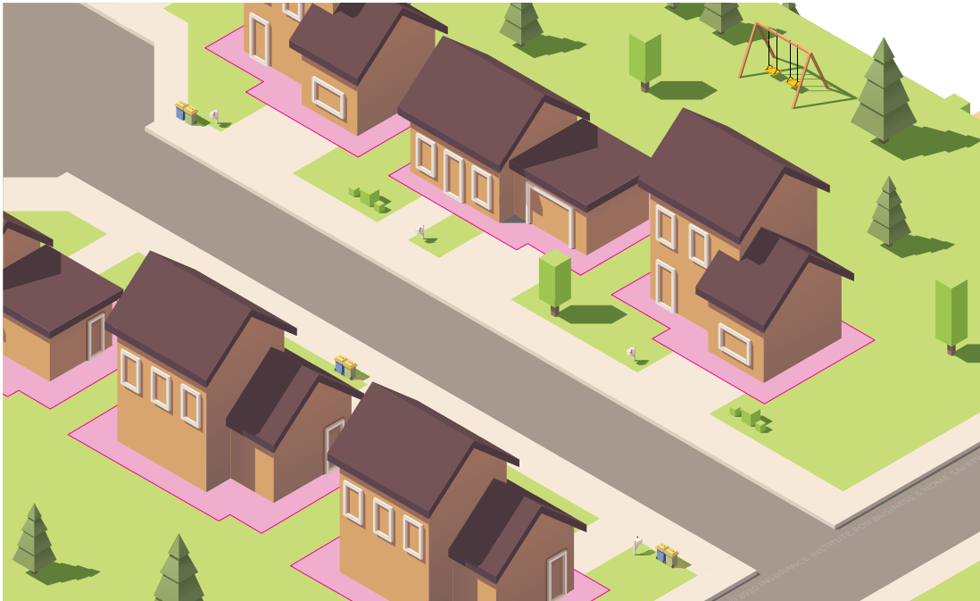
Figure 2. Idealized diagram of a typical suburban street and cul-de-sac. The pink 0-5 ft noncombustible zone is provided for reference.
