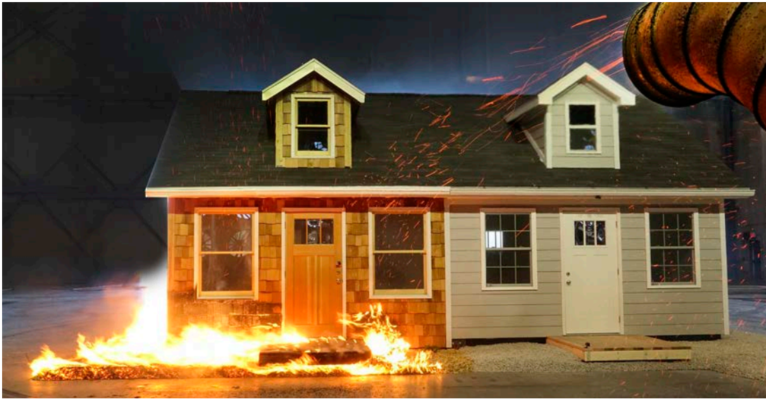
Figure 11. Importance of 0–5 ft noncombustible zone (home ignition zone) for a home under ember attack.
